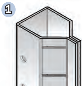
6-Bend Structural roll-formed vertical framing member
