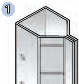
6-Bend Structural roll-formed vertical framing member
