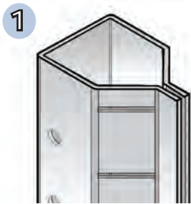
6-Bend Structural roll-formed vertical framing member
