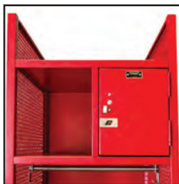
Optional Security Box uses Two heavy-duty 13 gauge 7-knuckle 3-1/2" hinges and a finger pull padlock hasp
